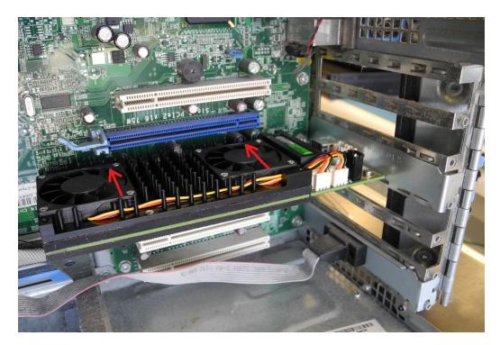
6. Secure the card hold-down bracket with a screw or other restraint, as appropriate in your computer.
