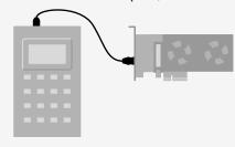
2. Luna PED Firmware 2.8.0 and newer is powered via the USB connection. If you are using Luna PED Firmware 2.7.1, connect it to power using the Luna PED DC power supply.
