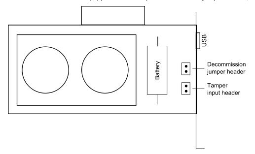
By default, short-circuiting the decommission jumper header decommissions the HSM. You can use the blade of a screwdriver, or other conductive tool to short-circuit the two pins of the decommission header, or you can connect a switch to the decommission header if desired. Power is not required to decommission the HSM, that is, you can decommission the HSM after removing it from the chassis.
