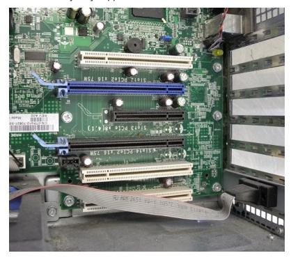
**5.** Insert the Luna PCIe HSM 7 card into the connector. It should go straight in – angling the card might cause it to bend. The card is properly seated when no portion of the gold-colored contacts of the card-edge protrudes above the connector socket.
